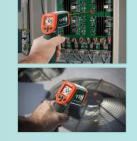
Compact non-contact InfraRed (IR) Thermometer measures up to 1112°F (600°C) with built-in laser pointer to identify target area and improve aim. Type K input allows for high temperature measurements up to 1832°F (1000°C). Builtin temperature sensor also measures Air Temperature. Adjustable emissivity feature allows for a higher accuracy when measuring temperature on various surfaces.
